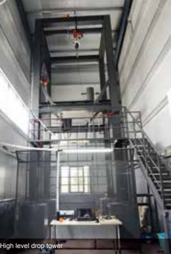
High level drop tower
